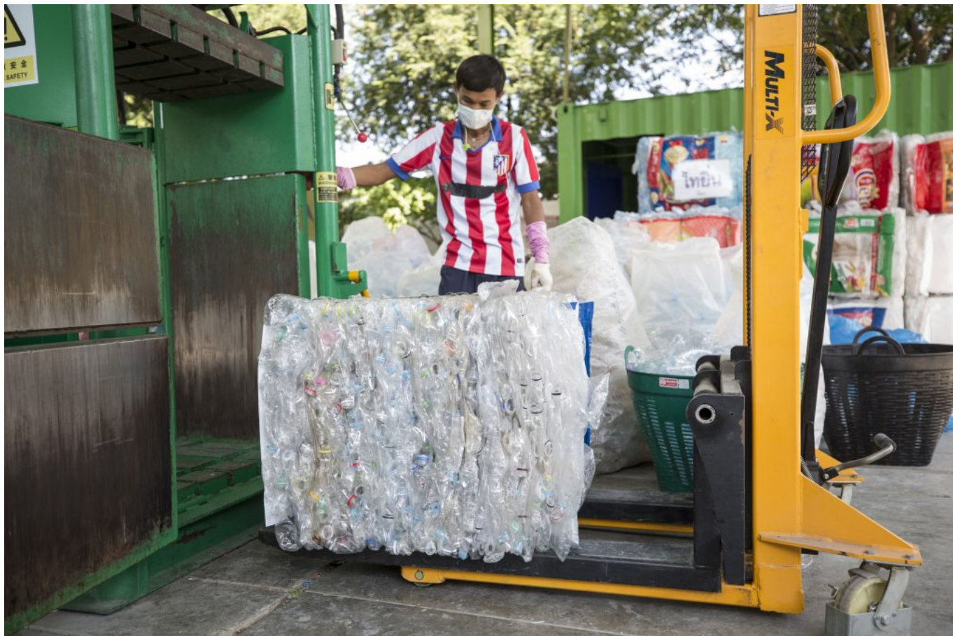
A volunteers empties donated plastic bottles, already separated and cleaned, in to a compacting machine that will produce a large 'bale' of crushed bottles. This will then be sent off to a factory for recycling and being made in to monks robes amongst other things.
